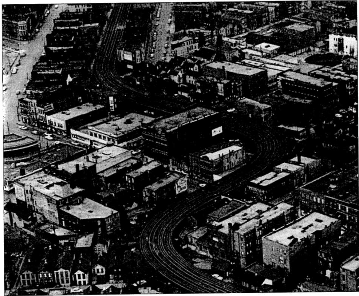
Above: Contrary to popular belief, the "L" was not designed to avoid the Yondorf Block and Hall. The track's weaving route, instead, was determined by existing alley rights-of-way, as seen in this detail from a 1958 photograph.
